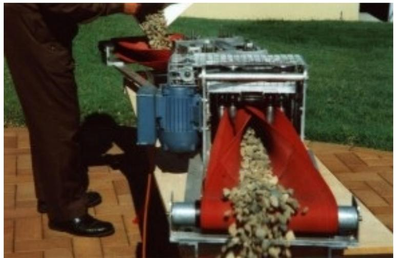
The CAP was initially designed for mining use where the idler bearing frame can be bolted to the side or the drive roof. Alternatively it may be supported by a trolley running on an overhead "I" beam, as is now commonly installed in coal mine development drives. The latter option means the CAP can be retracted and advanced from the tunnel face as soon as an I-beam extension is installed.
