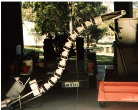
The photos show a bench test of fine phosphate sand material being conveyed at 70 degrees through two tight vertical curves. CAP equipment has the capacity to replace some bucket elevator applications.
