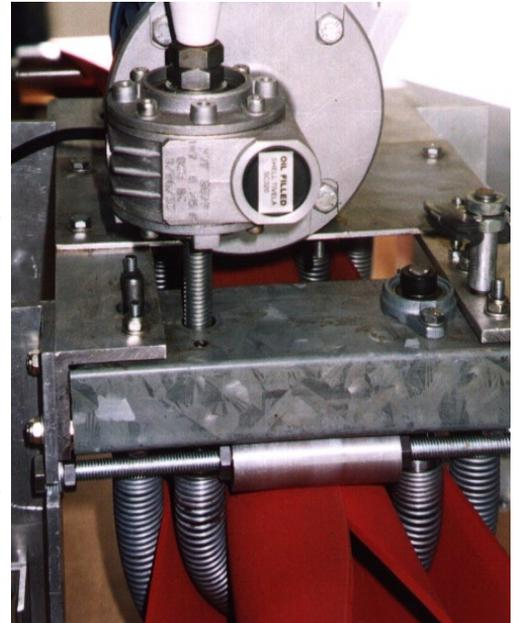
Our bench tests show the spring idler grips the belt very effectively when transferring spring torque to the conveyor. The action of the rotating spring simultaneously provides motive power to both the forward and return runs of the conveyor belt. This also allows a large single conveyor drive system to be replaced by a series of small units spread along the conveyor route, and linked in parallel.
