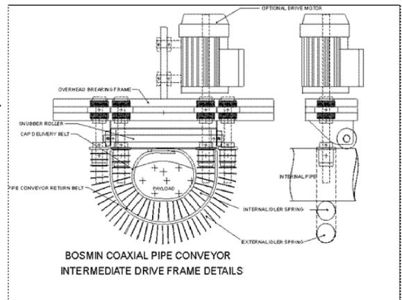
This critical design element allows for tight cornering with the CoAxial Pipe Conveyor (CAP), and is a distinct advantage over the very stiff specialised belts used with existing tube conveyors. The CAP belt can be butt-joined using rubber adhesive compounds, making belt extension or belt repairs a relatively simple task.
