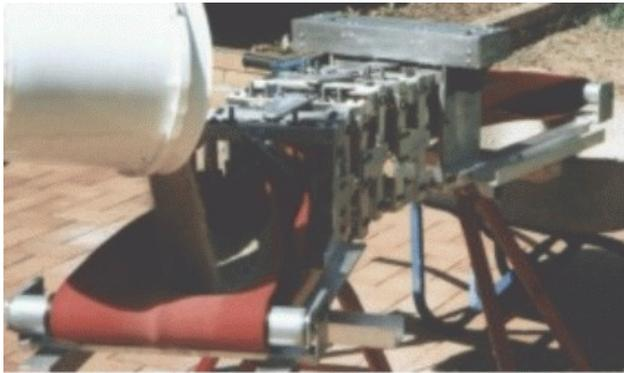
The CoAxial Pipe Conveyor is operating on a 26° turn at a 20:1 pipe diameter to curve radius.. The articulated frames permit tight vertical and horizontal curves. Fixed CAP installations do not require the articulated frame structure, only support for the bearing mounts.
