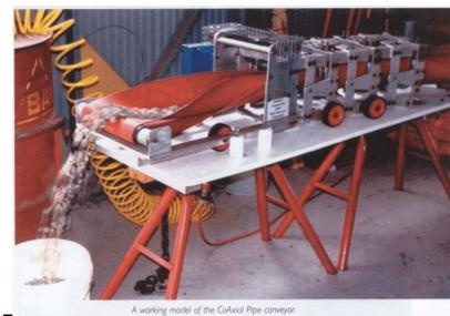
A working model of the CAP (Continuous Air Pipe) conveyor.
